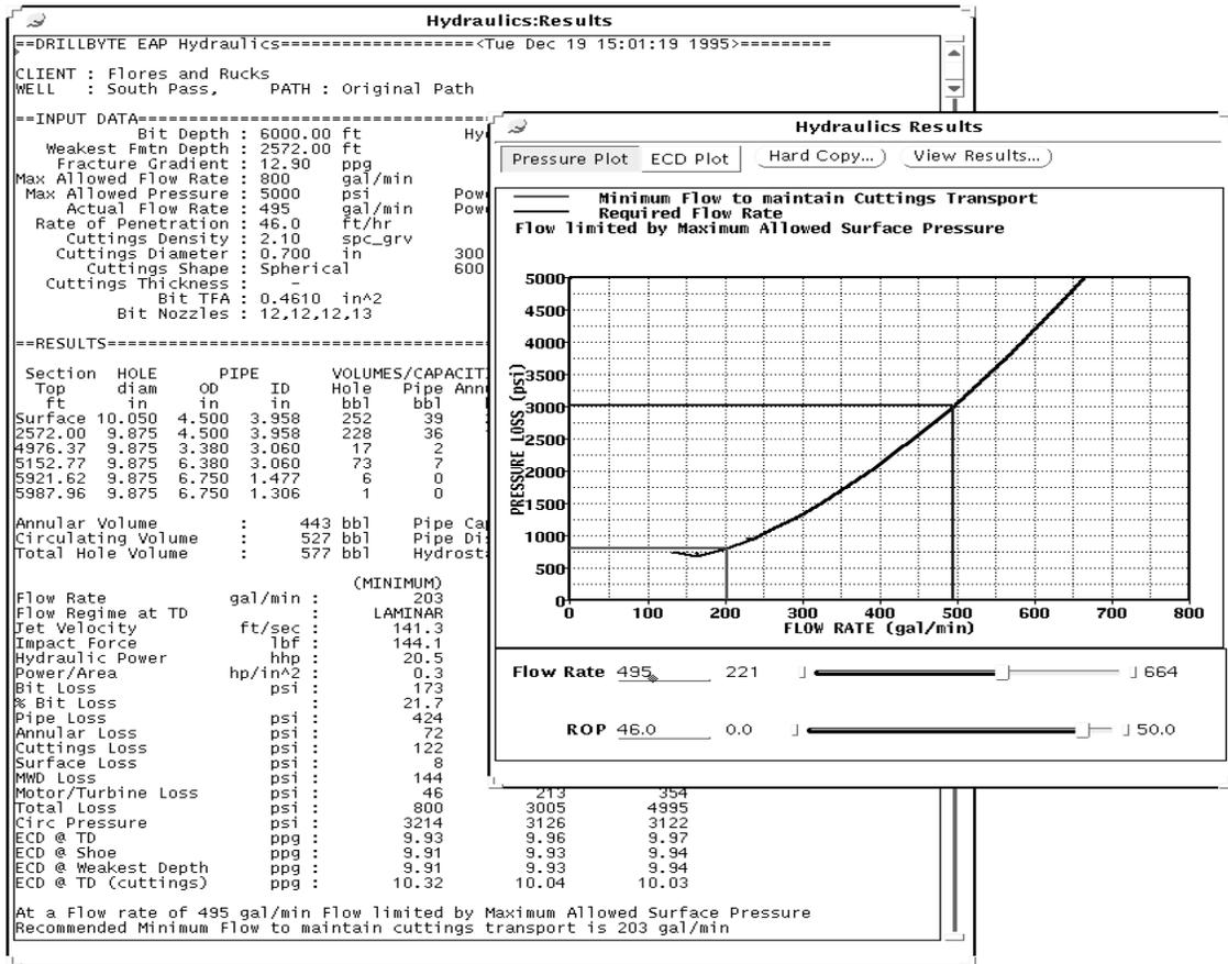
Figure E-5: Hydraulics Analysis Display — Screen shot from DrillByte
