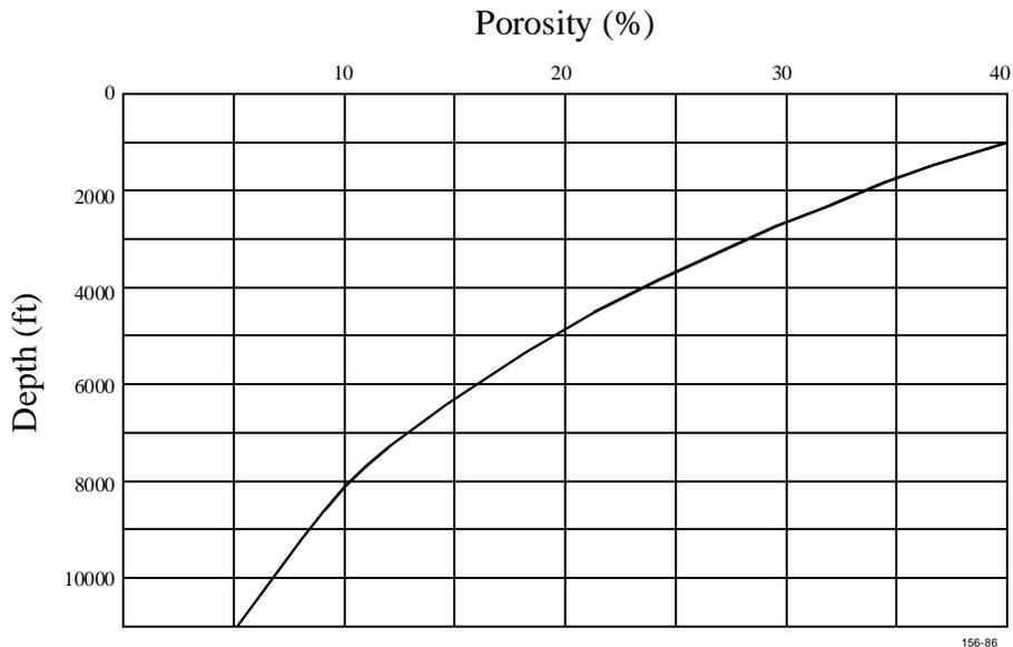
**Figure 2-3: Porosity/Depth relationship for a typical compacting clay sequence**
