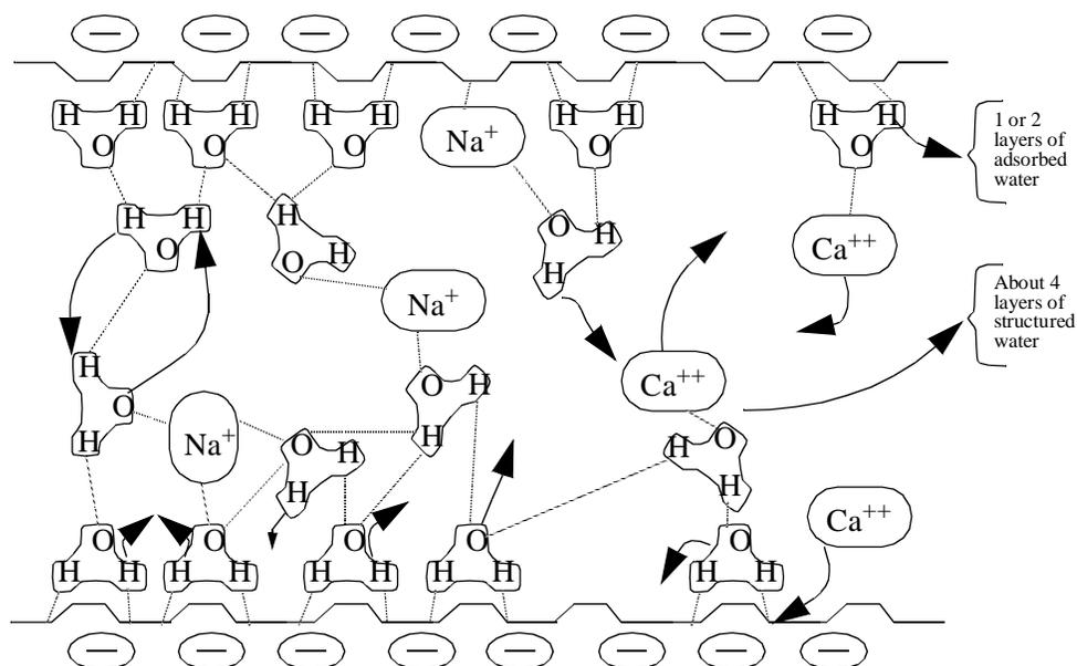
**Figure 2-8: Hydrogen bonded water and exchangeable cations**
