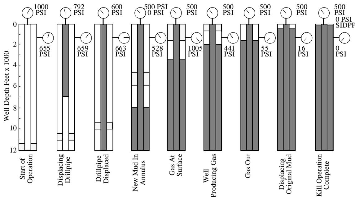
Figure 6-6: Shows diagrammatically the displacement of the original mud with kill mud, with example pressures, using the engineers method.
