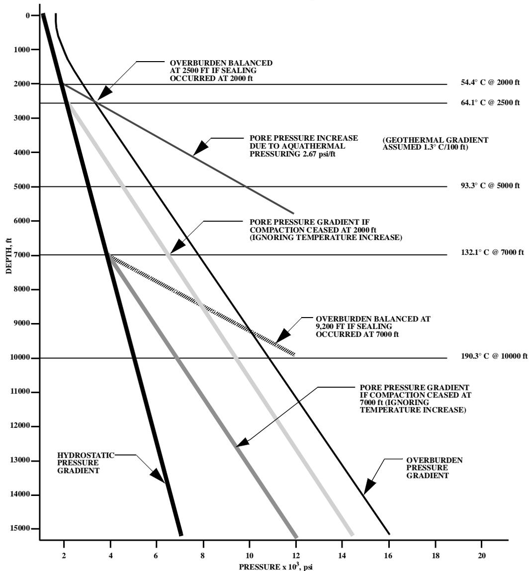
Figure 2-12: Pore pressure increases with geothermal gradient
