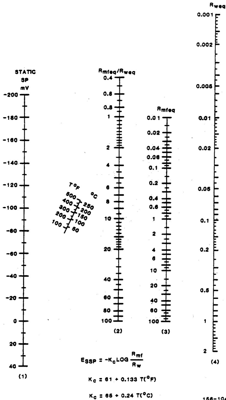
Figure C-5: Rweq determination from the SP (clean formations)
