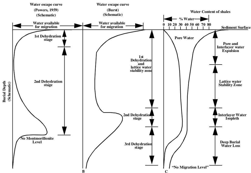
Figure 2-10: Hypothetical dehydration curves of Montmorillonite sediments with depth and temperature
