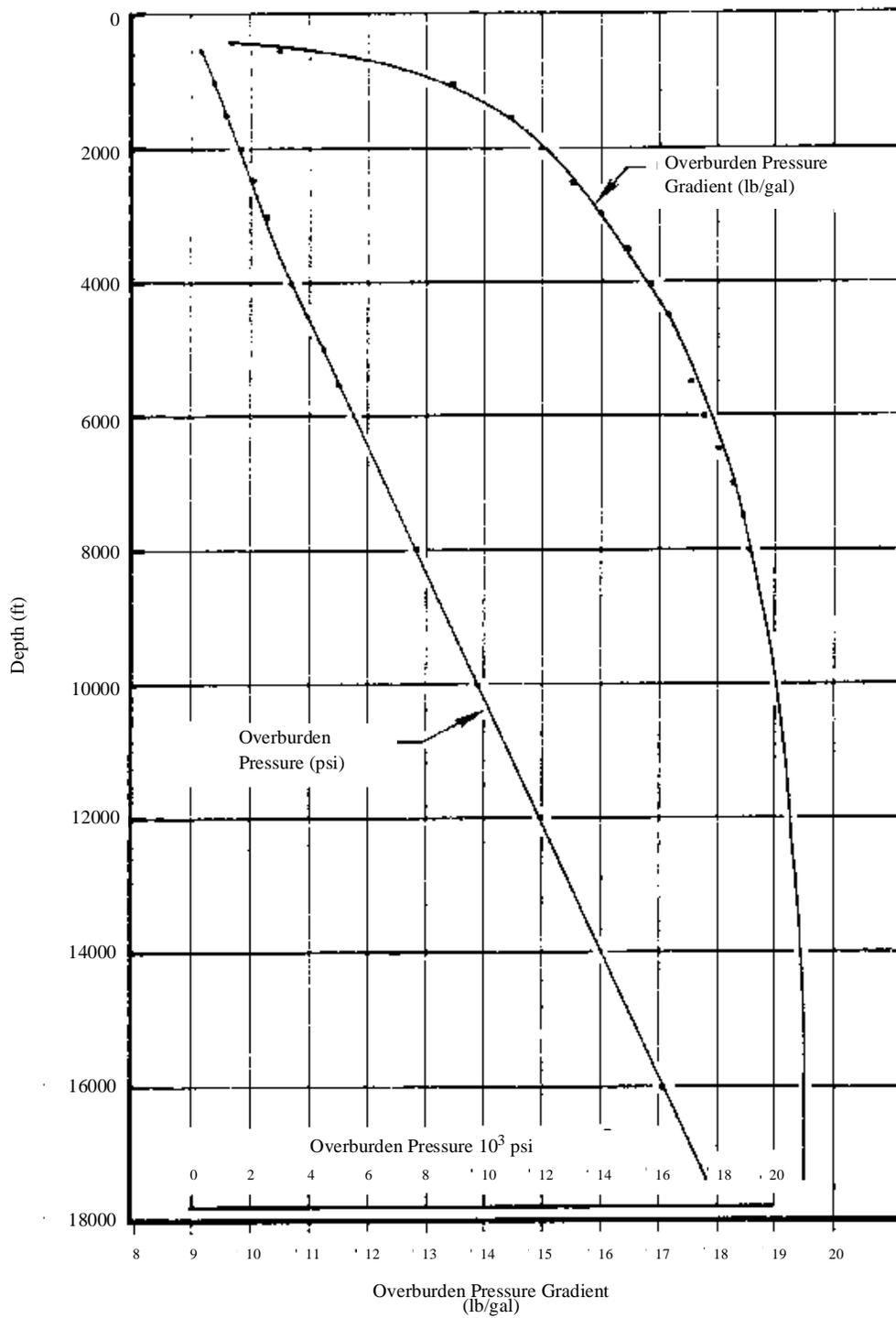
Figure 5-6: Typical overburden curve from an offshore well
