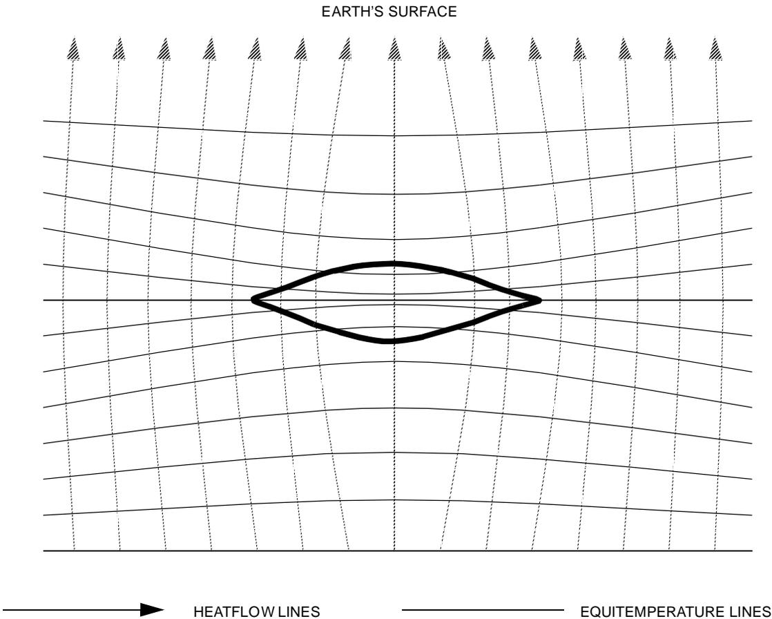
**Figure 4-15: Distribution of heat-flow and isotherms around an insulating (geopressed) zone**
