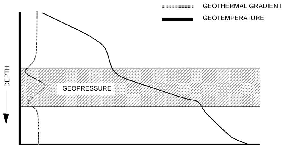
**Figure 4-16: Theoretical change of geothermal gradient through an insulating (high porosity/geopressured) zone**
