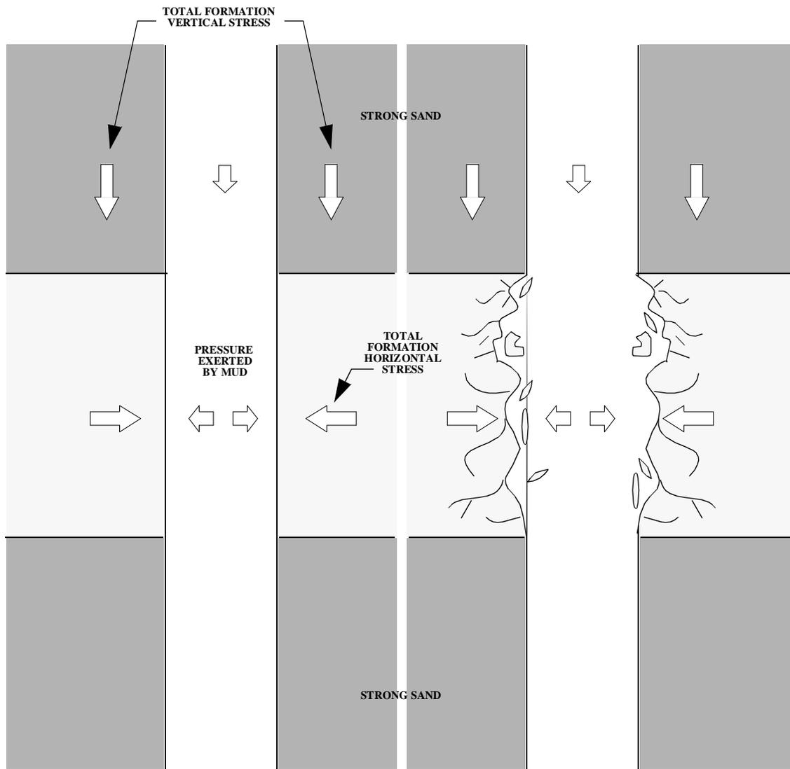
BOREHOLE WALL IS STABLE WHEN THE DIFFERENCE BETWEEN THE LATERAL STRESSES OF THE FORMATION AND THE LATERAL STRESS IN THE BOREHOLE IS LESS THAN THE STRENGTH OF THE WEAKEST FORMATION.
