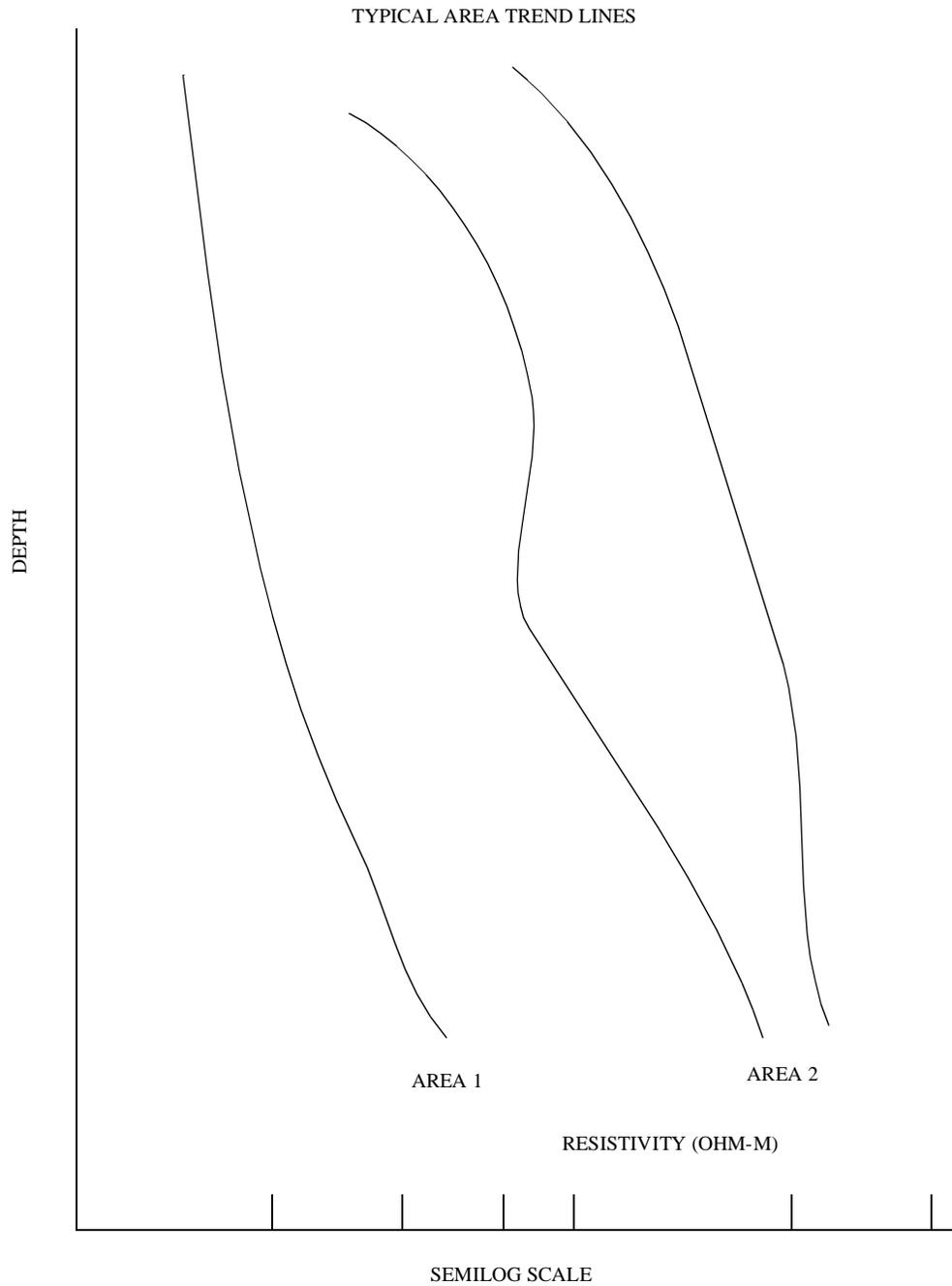
Figure 4-25: Formation resistivity typical area trend lines
