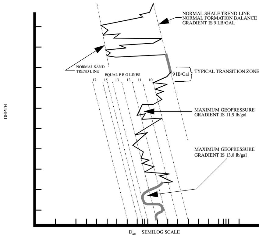
Figure 4-11: Example of the formation pore pressure gradients from the  $D_{xc}$  plot
