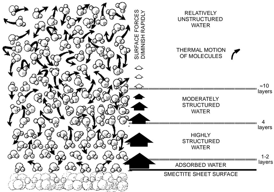
**Figure 2-9: Dynamic Structuring of water**
