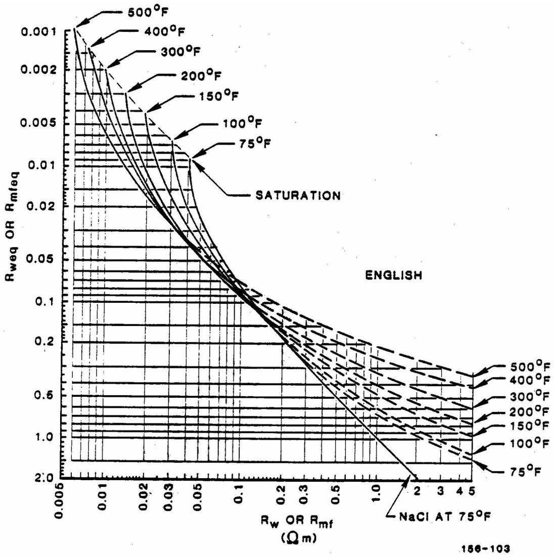
Figure C-4: Rw versus Rweq at formation temperature
