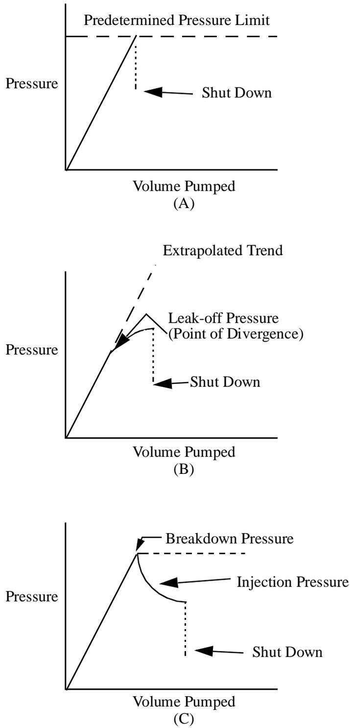
Figure 5-9: Leak-Off Test Pressure Limits
