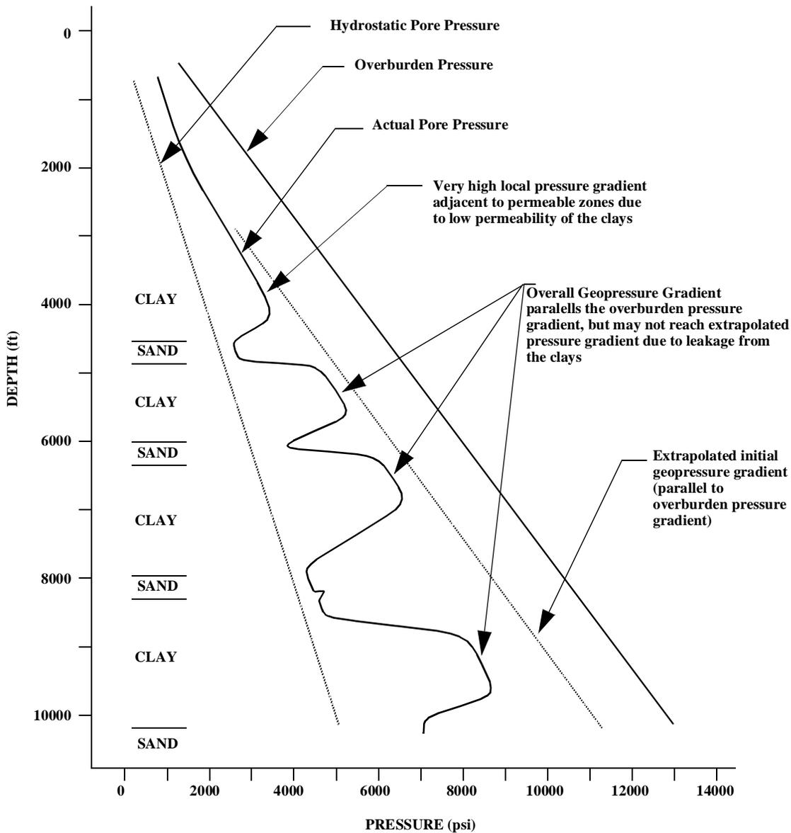
Figure 2-5: Typical Pore Pressure Depth plot of compaction disequilibrium geopressures
