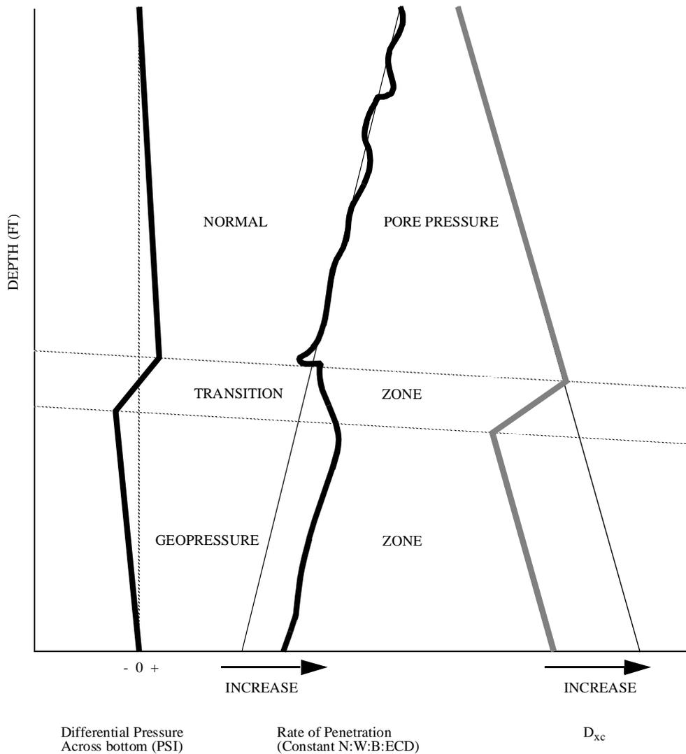
**Figure 4-9: Highly stylized curves showing typical response in transition and geopressed zones**
