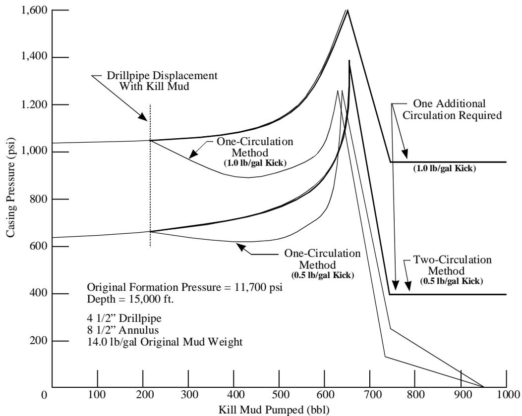
**Figure 6-1: Different surface pressures produced during the one and two circulation kill methods**
