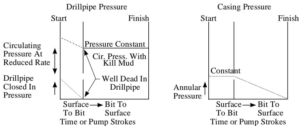
Figure 6-4: Second circulation during the drillers method.
