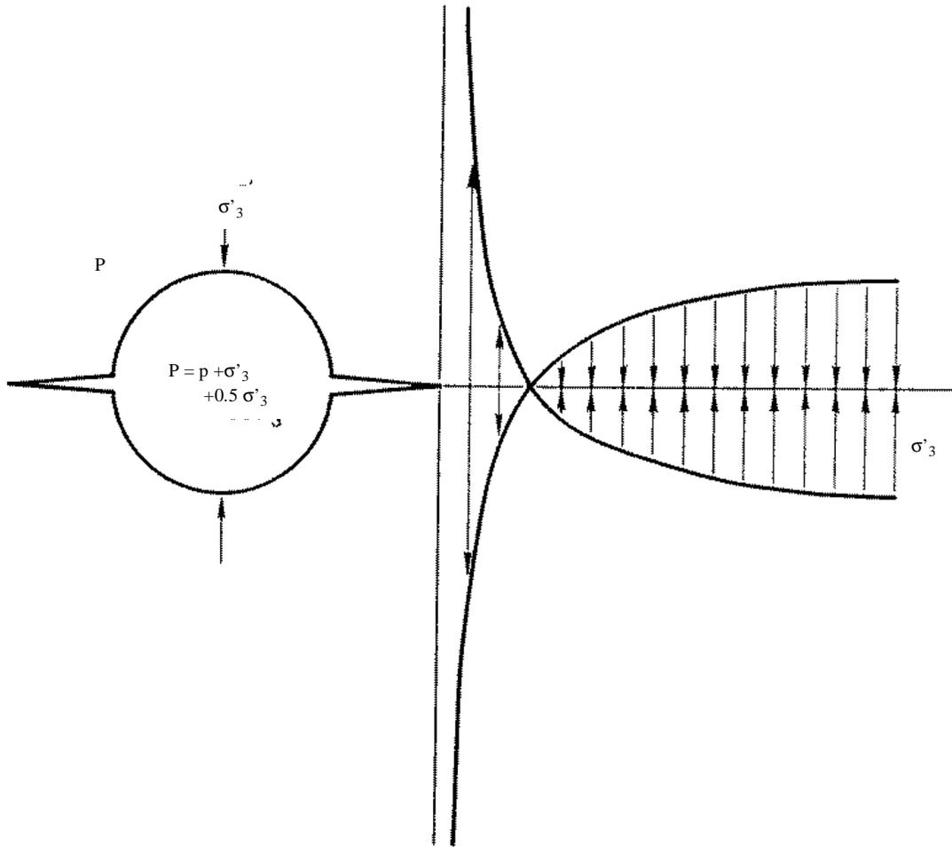
Figure 5-4: Tensile Stress produced at the tip of a crack
