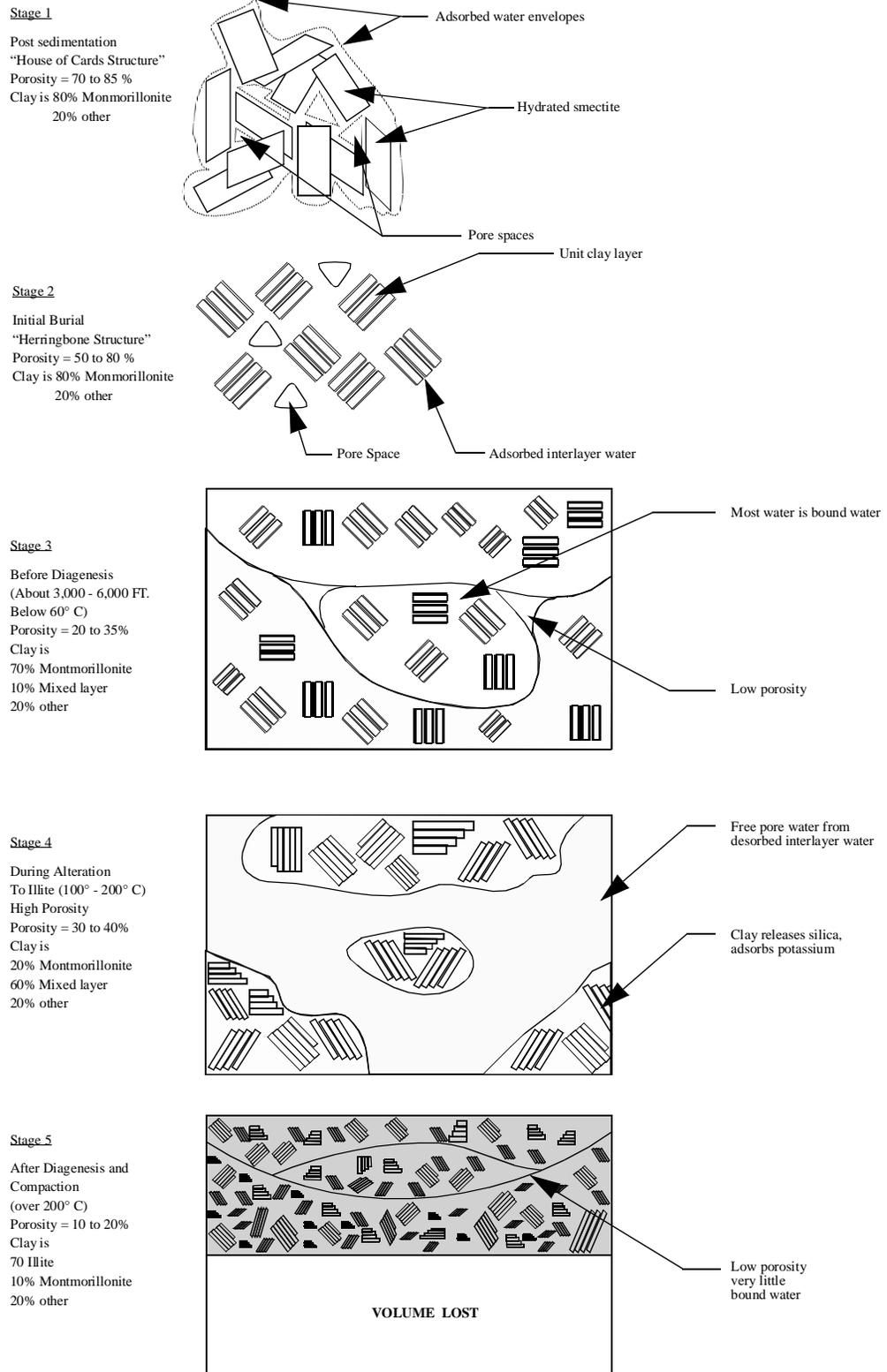
Figure 2-11: Diagenetic stages in the alteration of montmorillonite to illite
