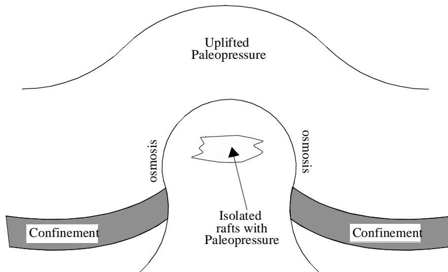
**Figure 2-13: Pore Pressure affected by Halokinesis**
