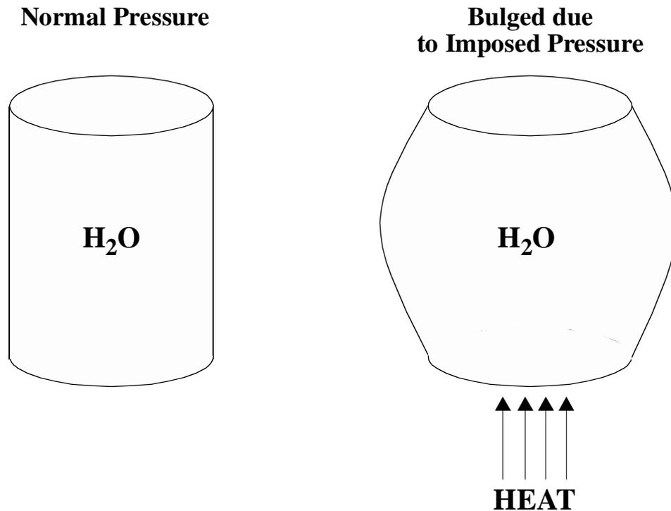
Figure 2-1: Imposed Pressure on a Cocoa Tin
