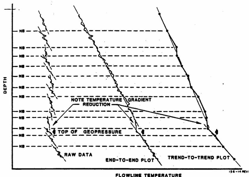
**Figure 4-18: Plots of flowline temperature, smoothed end-to-end plot and trend-to-trend**
