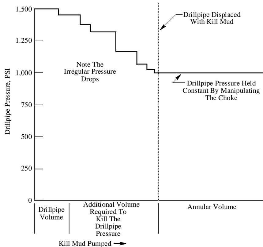
**Figure 6-7: Typical irregular drillpipe pressure reductions during concurrent method**
