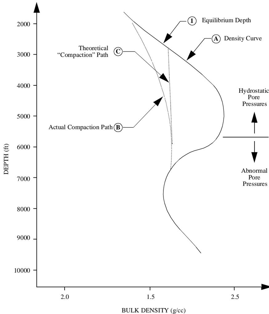
Figure 2-4: Bulk Density reversal in an abnormal pore pressure zone
