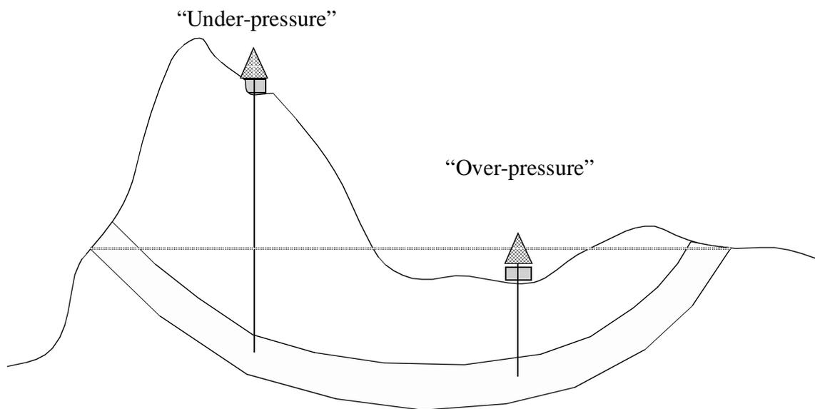
Figure 2-2: Piezometric Surface Effect on Pore Pressure
