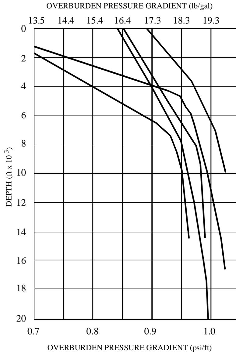
Figure 3-8: Typical Overburden Pressure Gradients
