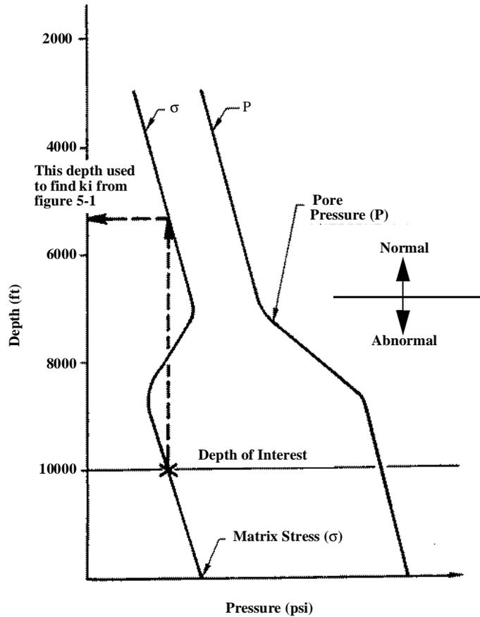
Figure 5-2: How  $k_i$  is obtained from the depth at which  $\sigma$  is normal
