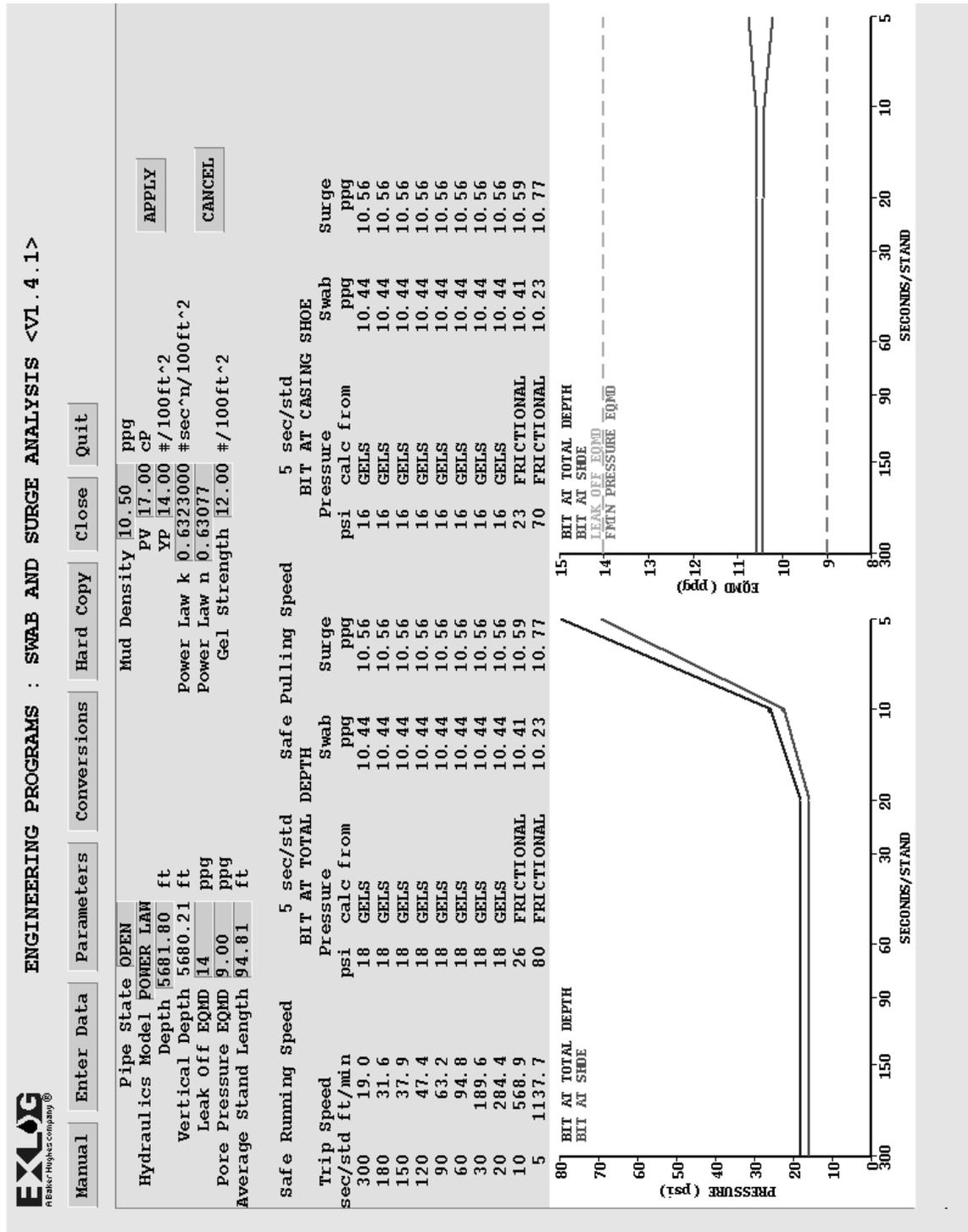
Figure 3-13: DrillByte Swab And Surge Analyses
