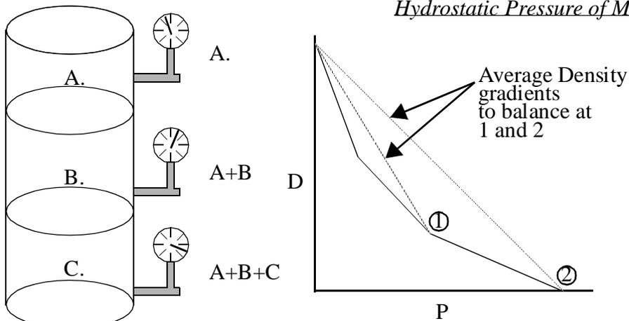
Figure 3-4: Hydrostatic Pressure of Single & Multiple Fluids
