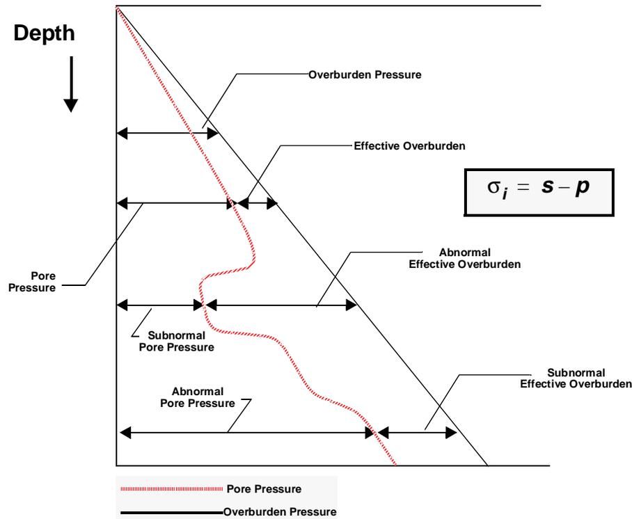
Figure 3-12: Effective overburden pressure in normal and geopressed formations
