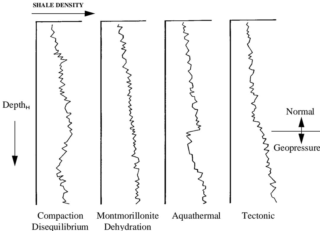
**Figure 4-12: Ideal clay density responses in geopressured zones caused by different mechanisms**
