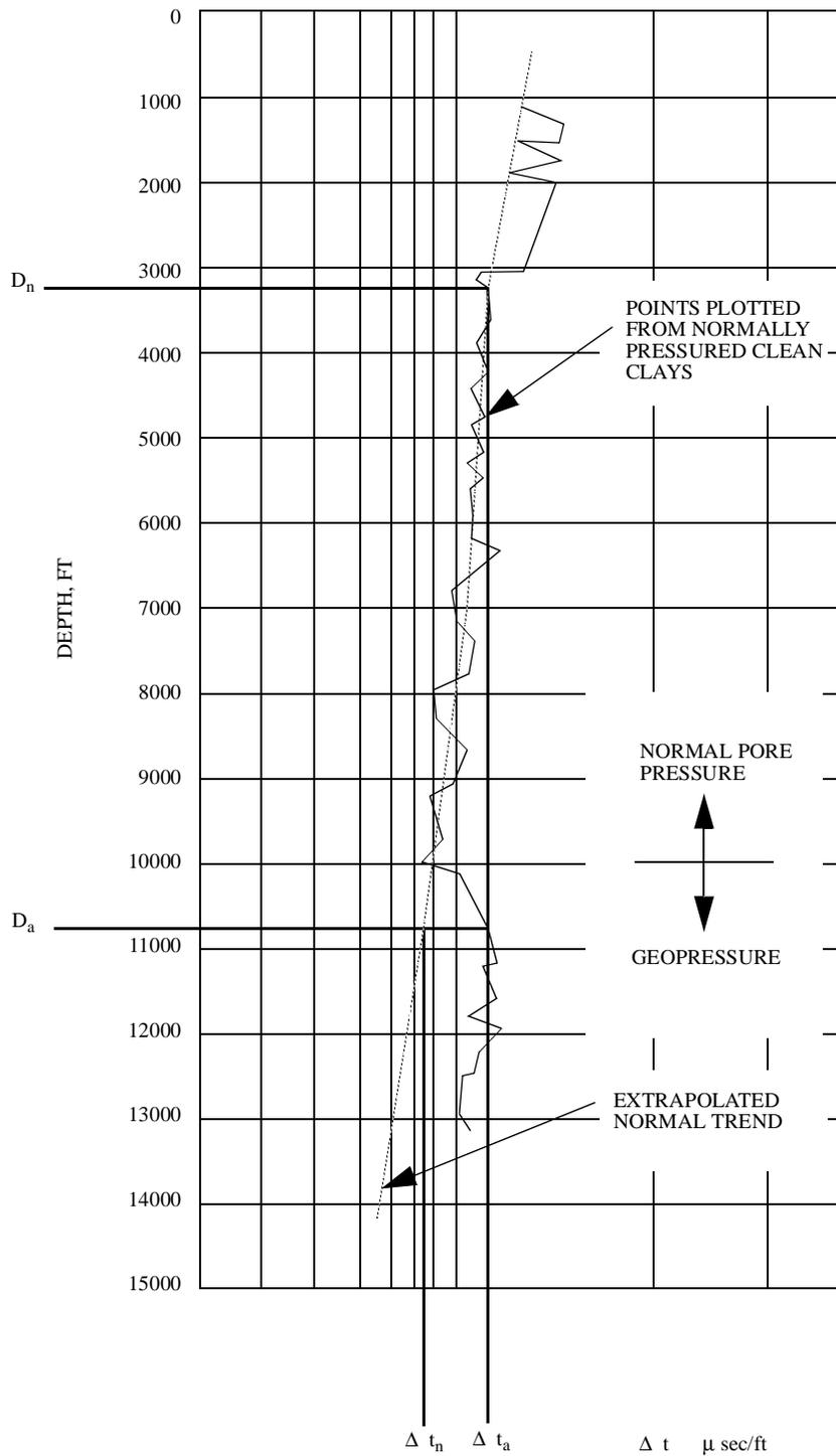
Figure 4-24: Geopressure evaluation using Equivalent Depth Method and sonic plot
