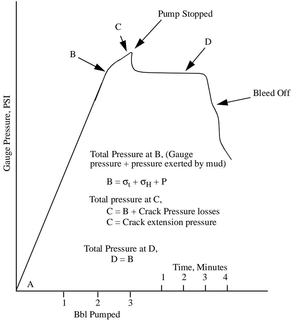
Figure 5-10: Typical Leak-Off Test Plot
