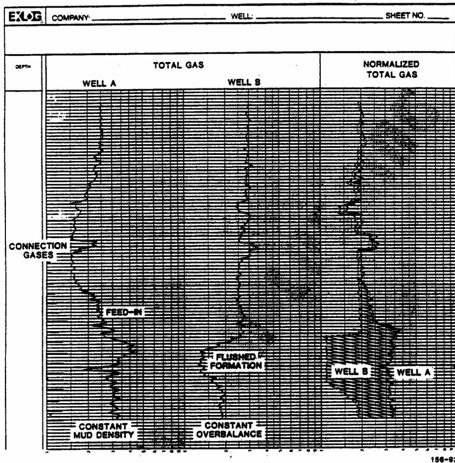
Figure 4-4: The effect of differential pressure on gas show magnitude
