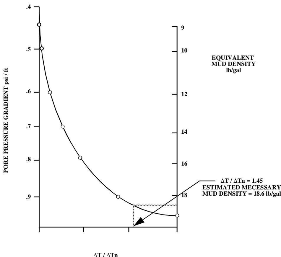
**Figure 4-3: Geopressure evaluation from interval transit time**
