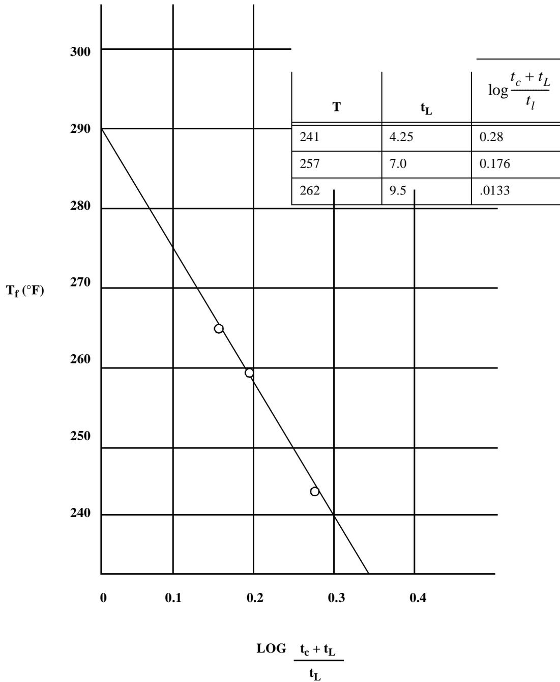
Figure 4-20: Horner-type plot of linear X-axis. Note less scatter in points
