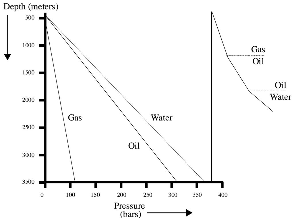
**Figure 3-3: Pressure Gradients of Water / Oil / Gas**
