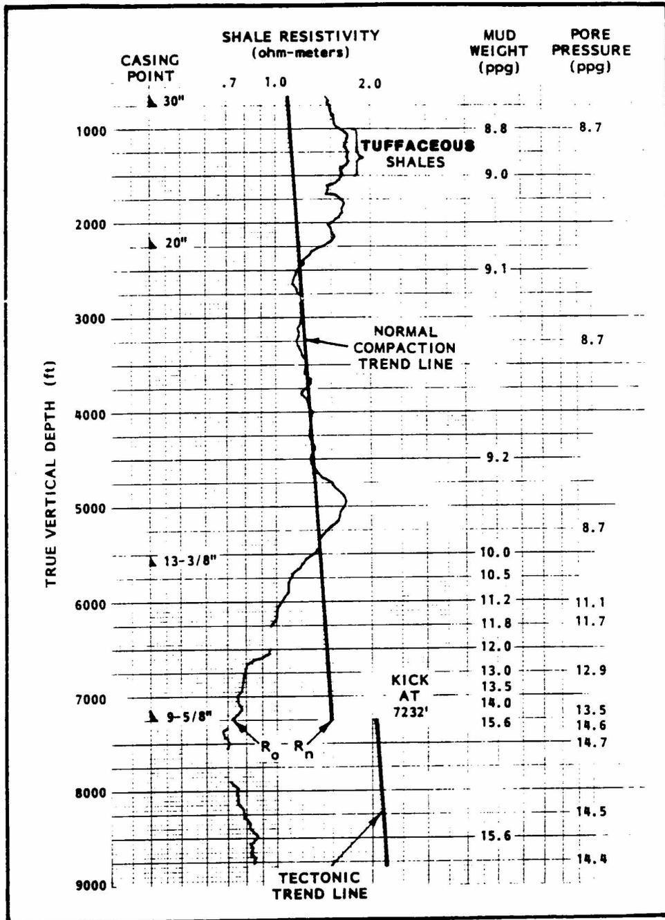
Note the normal compaction trend line and the tectonic trend line
