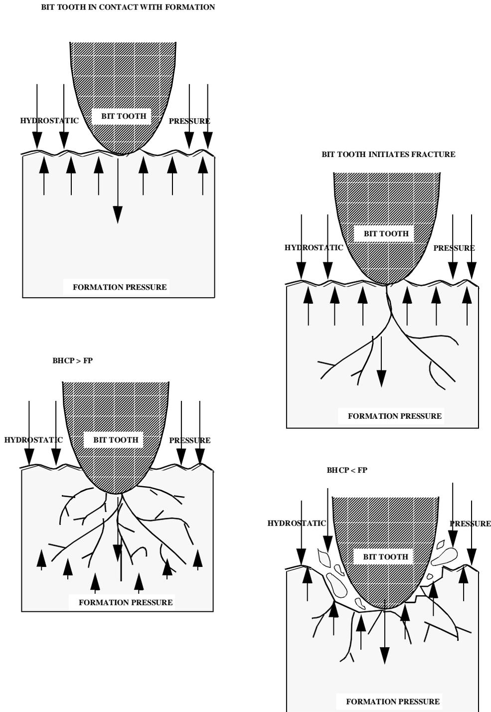
Figure 4-8: How drillability is affected by differential pressure in hard formations
