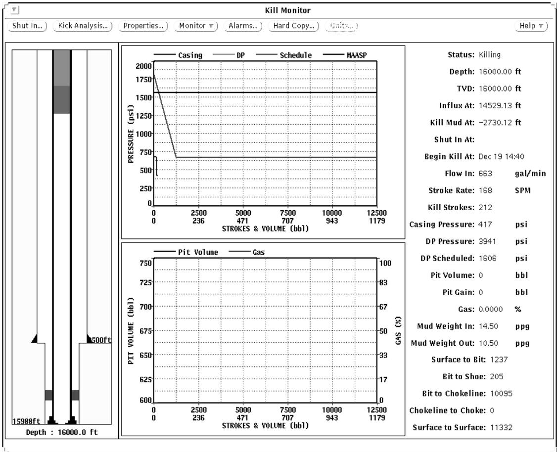
Figure E-3: Kill Monitor Display — Screen shot from DrillByte
