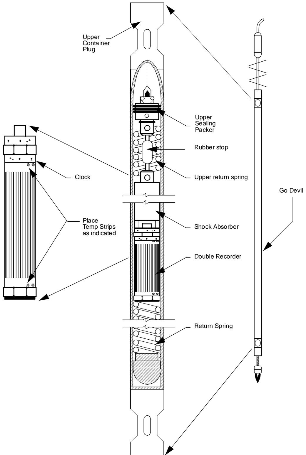
Figure 4-21: Location of Temperature Plates in deviation survey tool
