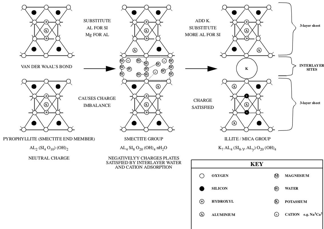
Figure 2-7: Changes in ionic substitution in three-layered sheets
