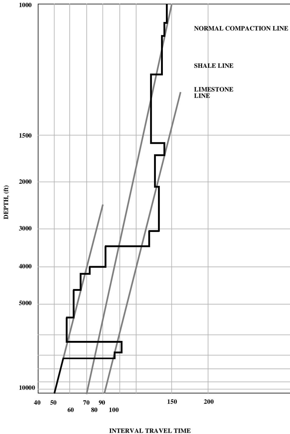
Figure 4-1: Interval transit time variations with compaction and lithology
