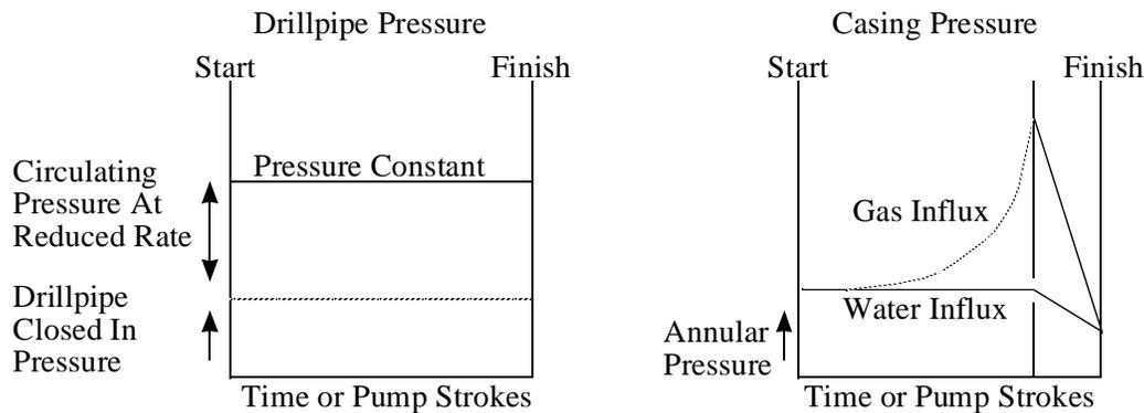
Figure 6-3: First circulation pressures during the drillers method.
