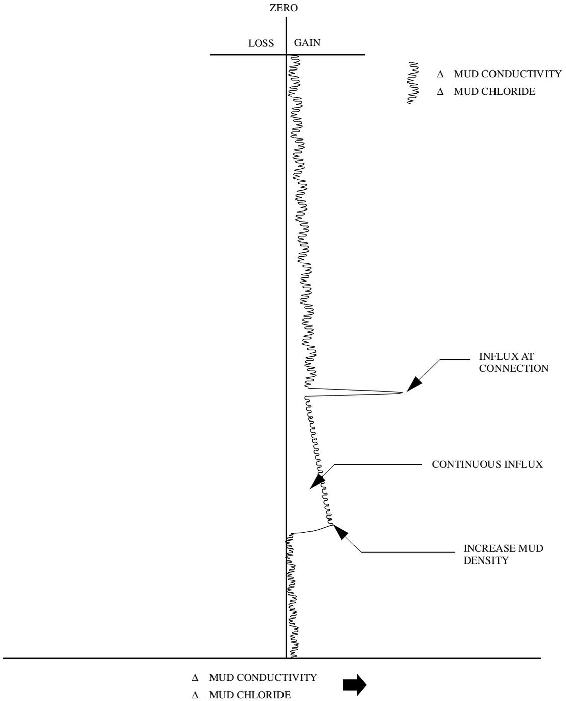
Figure 4-22: Differential mud conductivity and delta chloride log
