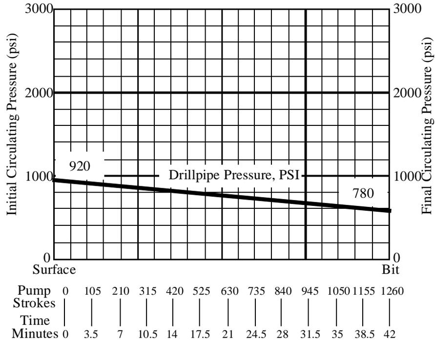
Figure 6-2: Drillpipe/pressure plot when kill mud is pumped down the drillpipe
