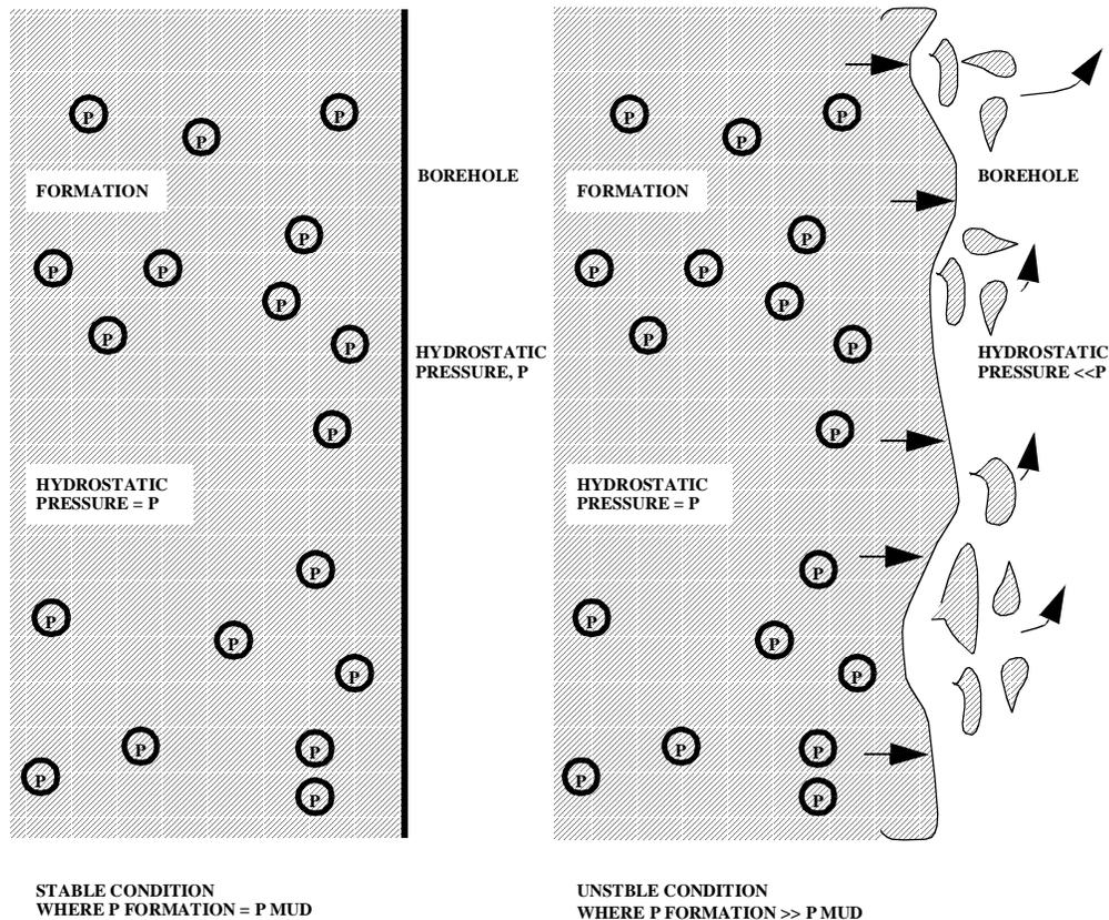
Figure 4-5: Cavings produced due to underbalanced drilling
