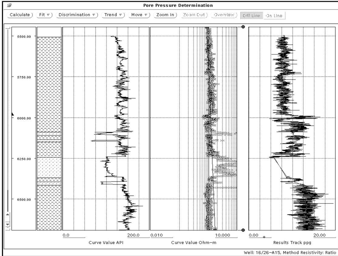
Figure E-2: GeoPress Pore Pressure Analysis — Screen shot from DrillByte
