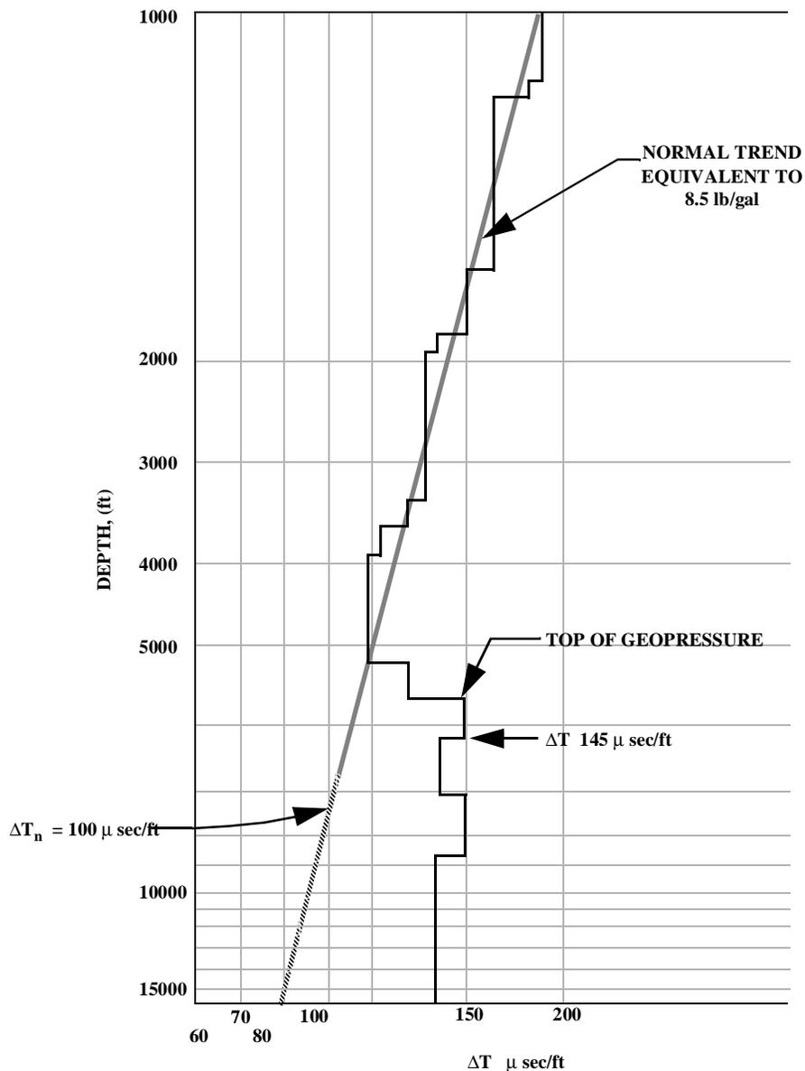
Figure 4-2: Interval transit time variation with pore pressure
