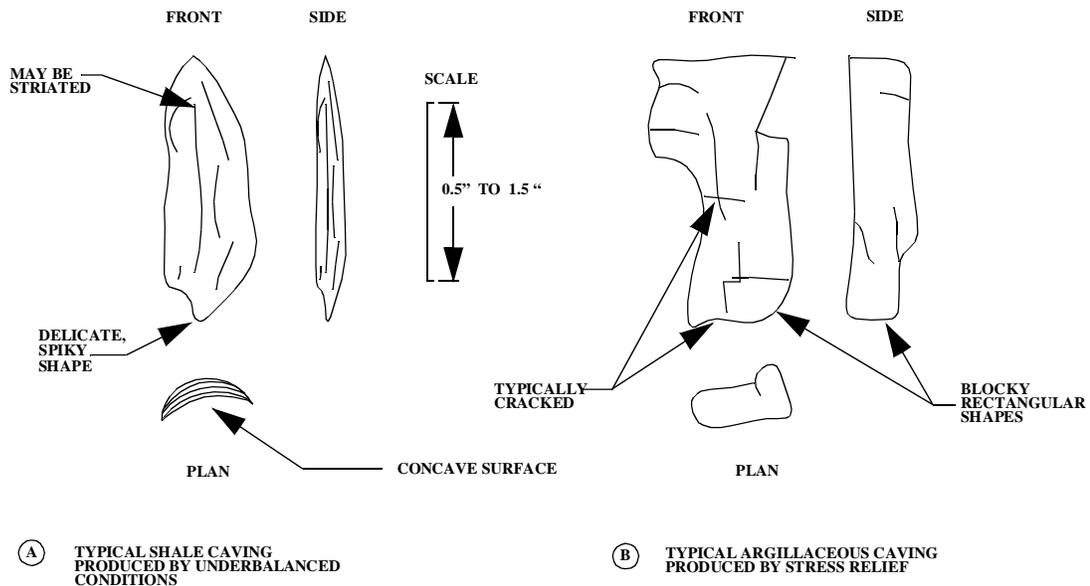
**Figure 4-7: Typical cavings produced by underbalance and stress relief**
