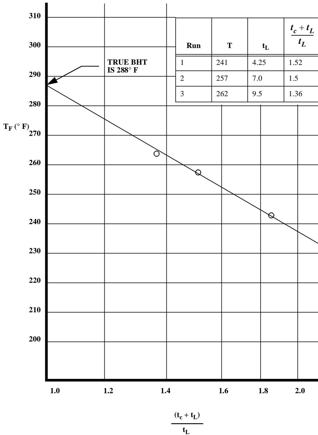
Figure 4-19: Horner-type plot for graphic solution of true bottomhole temperature
