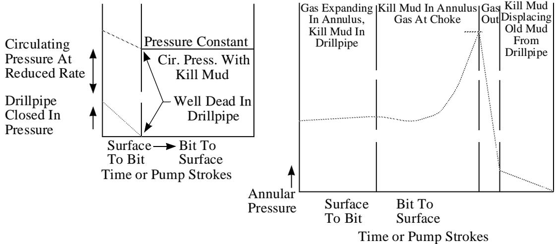
Figure 6-5: Drillpipe and annular pressure curves during the engineer's kill method
