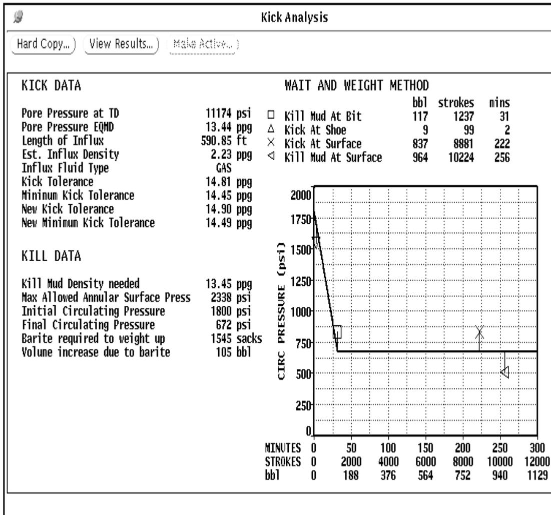
Figure E-4: Kick Analysis Display — Screen shot from DrillByte
