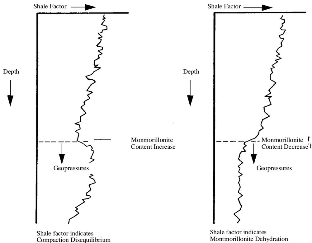
**Figure 4-14: Shale factor response in geopressures, caused by compaction disequilibrium or montmorillonite dehydration**
