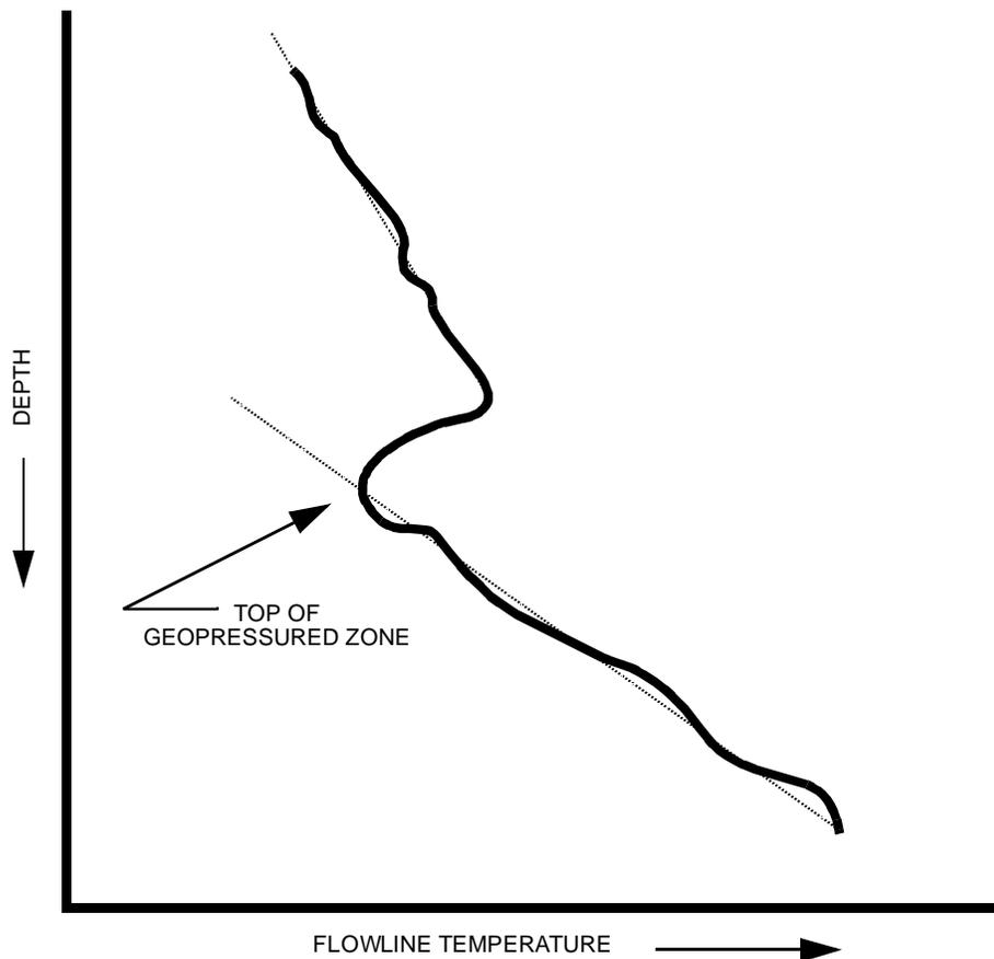
**Figure 4-17: Expected flowline temperature response on drilling through a geopressured interval**
